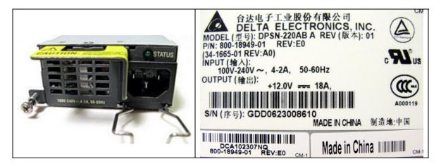
This is a universal AC input (100-240V) modular (plug in) 220W supply that outputs a nominal 12VDC at up to 18A. It has a standard IEC line cord connector (with plug retainer) and green status light (when operating). There is no fan inside the unit, but forced air (from within the cabinet) to exhaust the supply is a good idea above 10A to control heat build-up.
